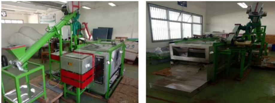
Figure 5: The Result of Designed Cassava Flour Processing Machine.
